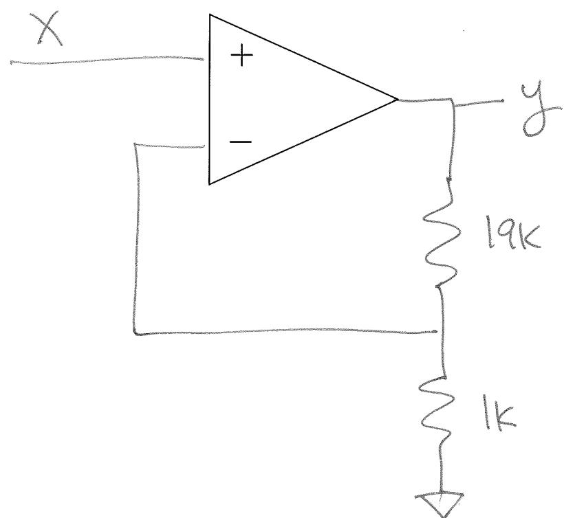
2) Design a circuit with a gain of +20 and an offset of +10V
