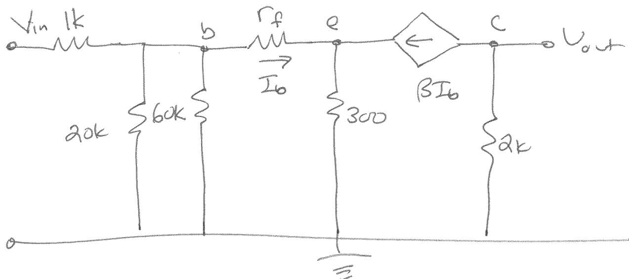
2) Draw the small-signal model (AC circuit) for the following common-base amplifier. Assume
