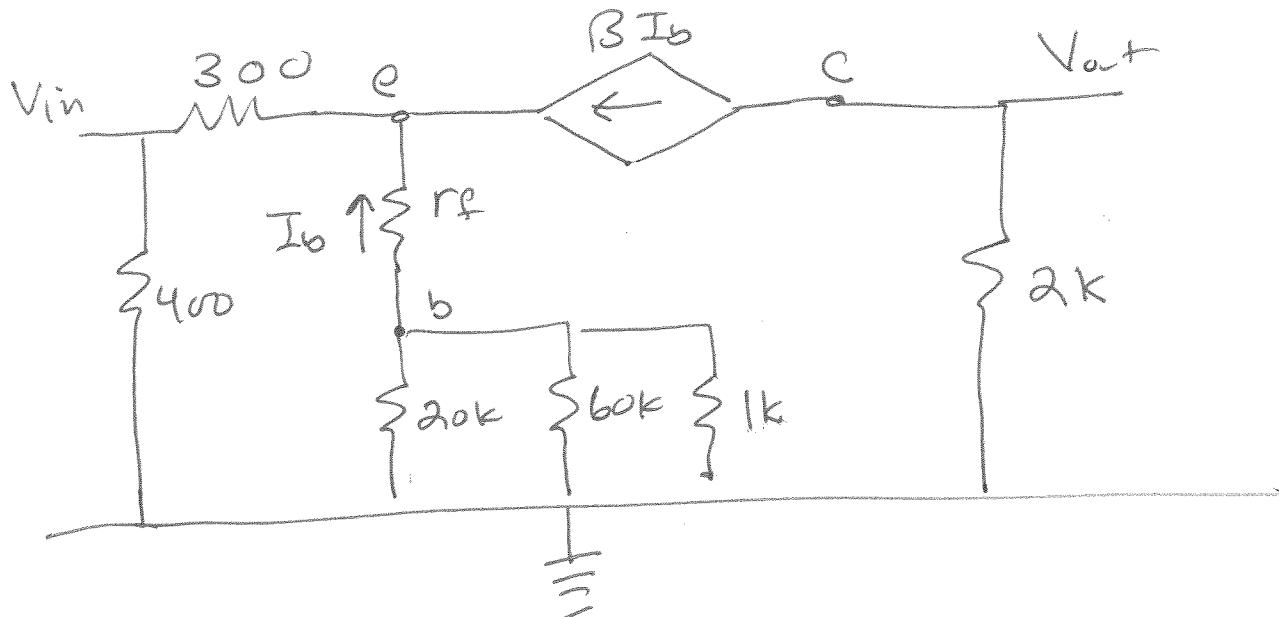
3) Determine the 2-port parameters for the following common-emitter amplifier:
