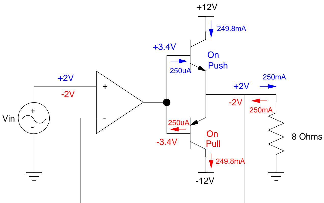
6) Simulation: Check your analysis in PartSim at Vin = +2V and -2V
