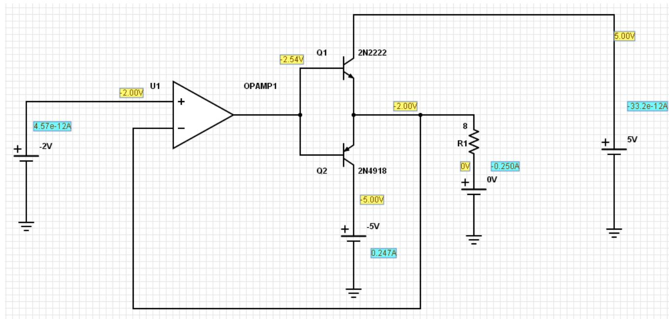
7) Lab: Build your circuit and measure the voltages at Vin = +2V and Vin = -2V.
