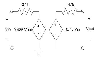
Rin: Short Vout. Measure the voltage at the input  $R_{in} = 100 + 300 ||400$
