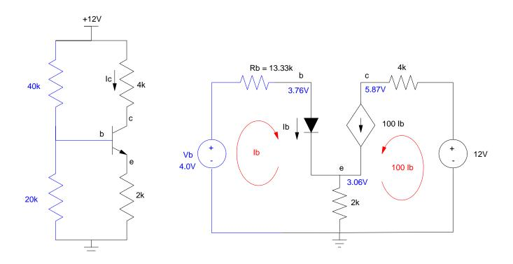
First, redraw the circuit using the Thevenin equivalent for the 40k & 20k resistor (shown in blue)
