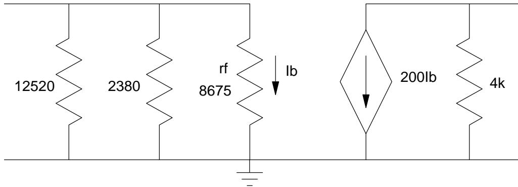
3b) Determine the 2-port model for this amplifier in a CE configuration.
