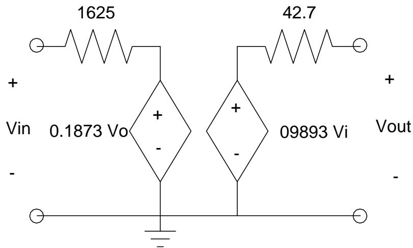
6) Determine the 2-port model for a 4-stage amplifier:
