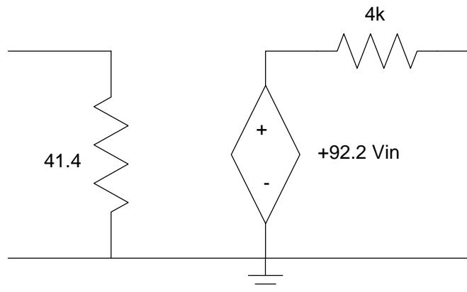
5a) Draw the small-signal model for your circuit of problem #2 when set up as a common collector (CC) configuration
