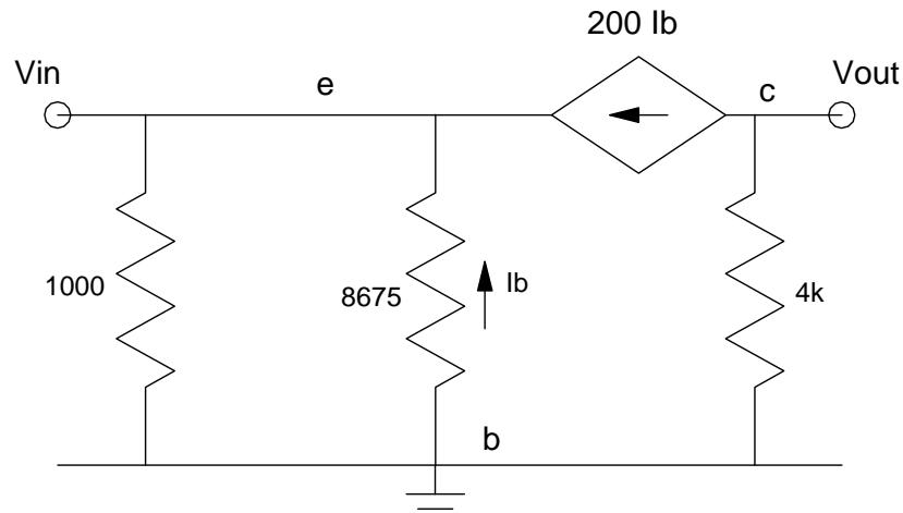
4b) Determine the 2-port model for this amplifier in a CB configuration.
