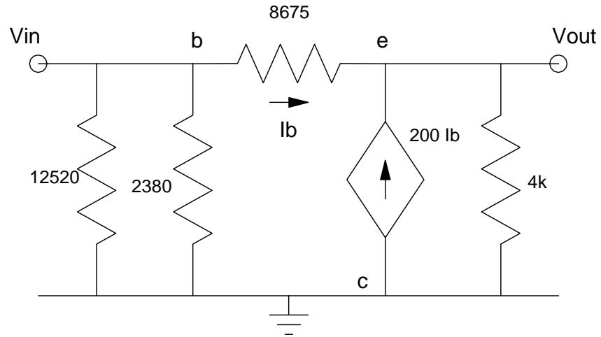
5b) Determine the 2-port model for this amplifier in a CC configuration.
