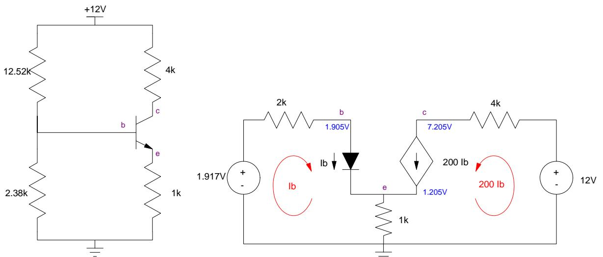
3a) Draw the small-signal model for your circuit of problem #2 when set up as a common emitter (CE) configuration
