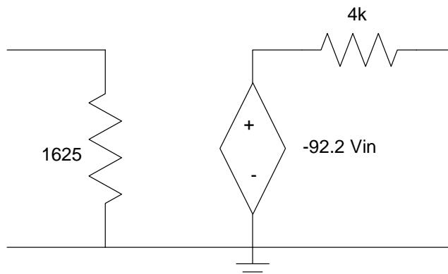
4a) Draw the small-signal model for your circuit of problem #2 when set up as a common base (CB) configuration
