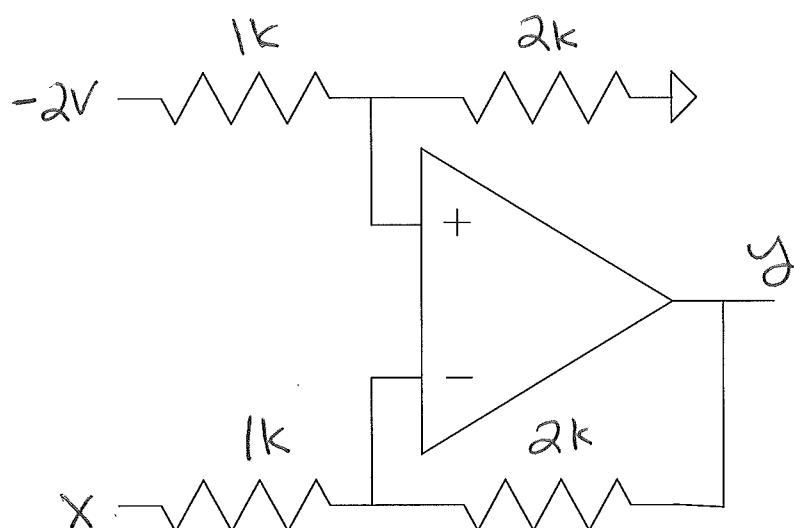
5) Determine the voltges for the following op-amp circuit.
