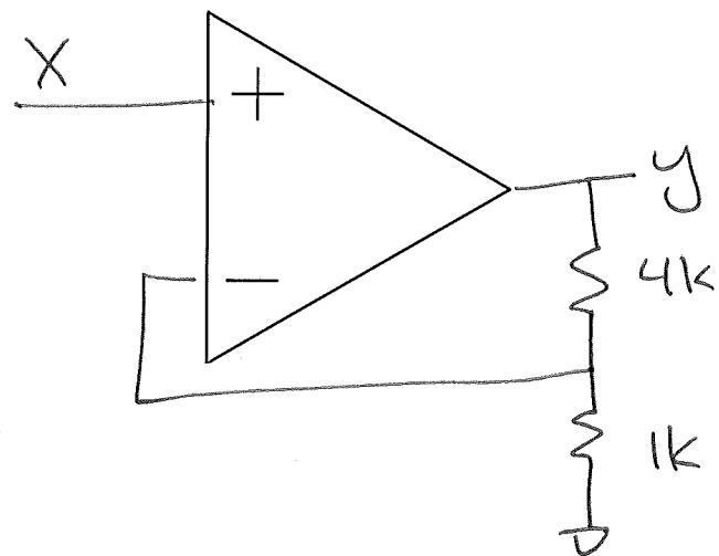
3b) Design an op-amp circuit with a gain of -5
