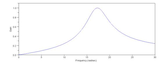
2b) Find the frequency, w, which results in the gain being a maximum (resonance):
