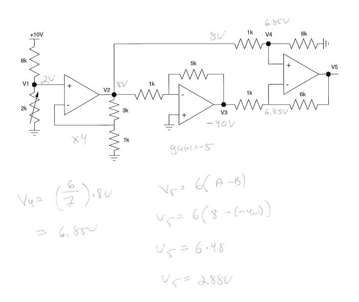
5) The voltage across a votlage divider is shown below. Determine a calibration function
