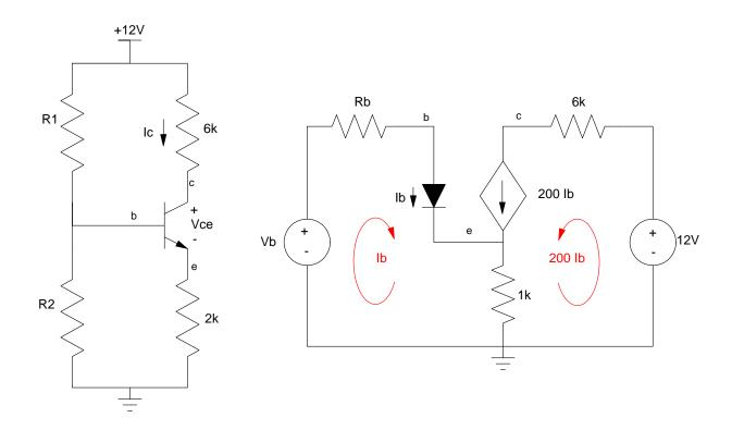
3) Small Signal Model. Draw the small signal model for the following amplifier. Assume
