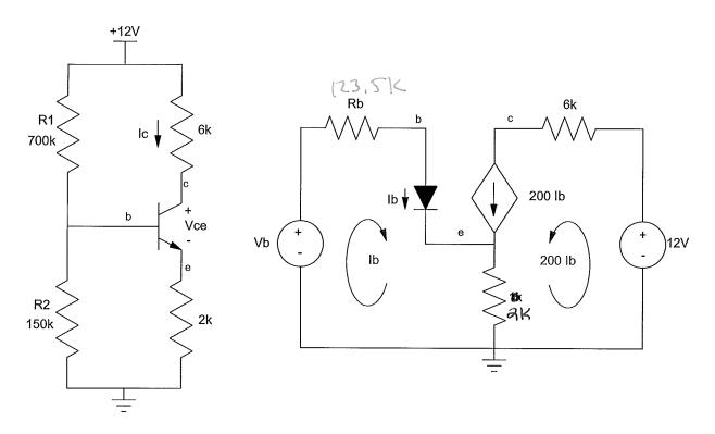
$$R_{b} = 700 \text{k} | 180 \text{k} = 123.5 \text{k}$$
