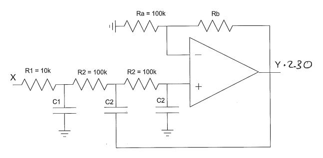
$$Y = \left(\frac{\left(\frac{1}{R_{1}C_{1}}\right)}{s + \left(\frac{1}{R_{1}C_{1}}\right)}\right) \left(\frac{k\left(\frac{1}{R_{2}C_{2}}\right)^{2}}{s^{2} + \left(\frac{3-k}{RC}\right)s + \left(\frac{1}{RC}\right)^{2}}\right) X \qquad k = 1 + \frac{R_{b}}{R_{a}}$$
