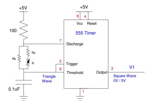
5 point Bonus! Build this circuit replacing the linearizing circuit with the thermistor in your lab kit. Measure the frequency resulting from placing the thermistor in
