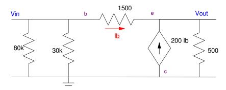
5) Determine the 2-port model for the following circuit
