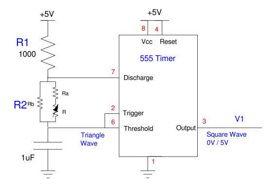
5 point Bonus! Build this circuit replacing the linearizing circuit with the thermistor in your lab kit. Measure the frequency resulting from placing the thermistor in
