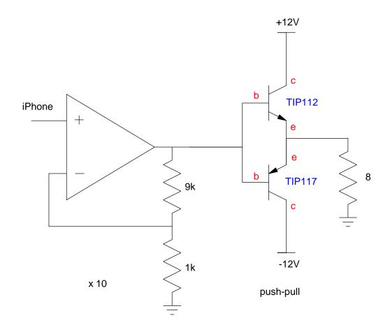
2) Design a push-pull amplifier without crossover distortion to amplify the output of an iPhone
