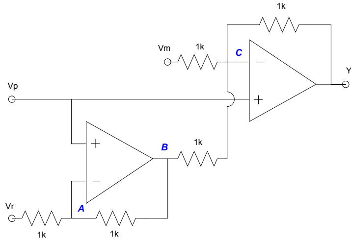
You need to write four equations for the four unknown voltage nodes (A, B, C, Y)
