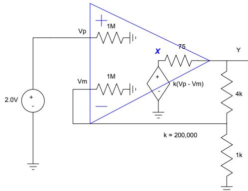
You need four equations for four voltage nodes: Vp, Vm, Y, X,
