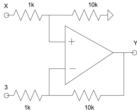
5) Instrumentation Amplifier (take 2). Design a circuit to implement the following:
