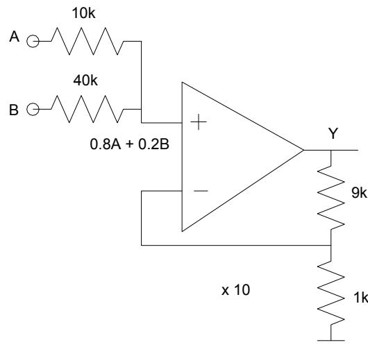
4) Instrumentation Amplifier. Design a circuit to implement the following:
