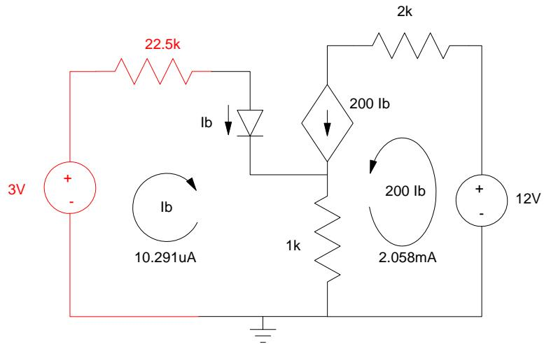
First, redraw the circuit using the Thevenin equivalent for R<sub>1</sub> and R<sub>2</sub>
