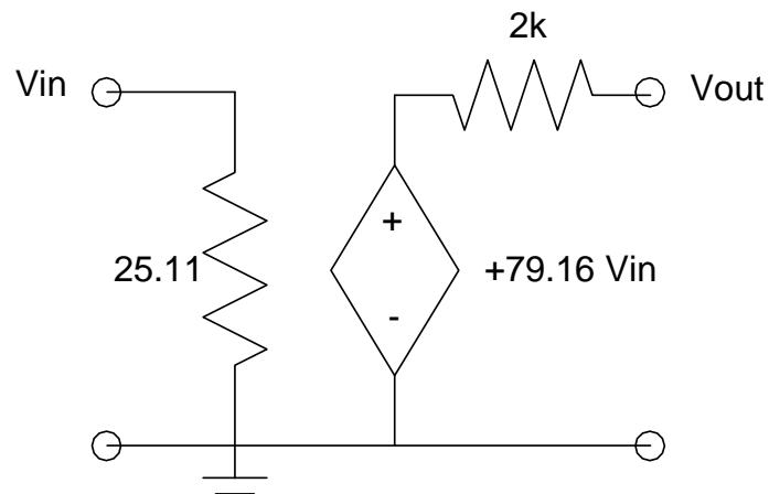
4) Find the 2-port model as a common-collector configuration
