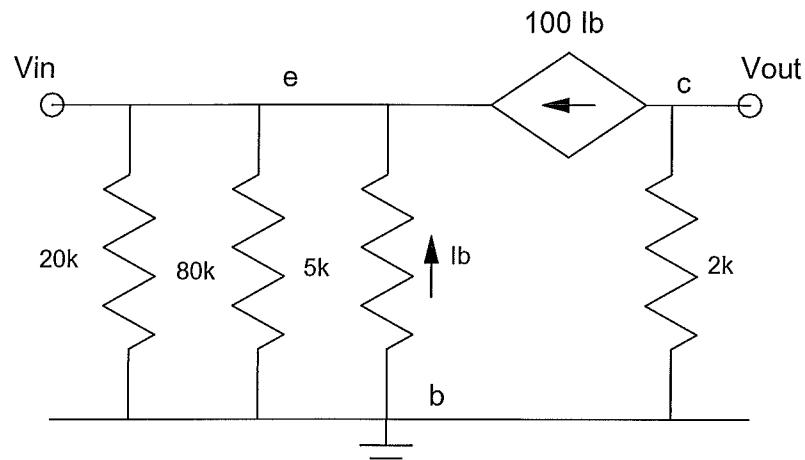
$$R_{in} = 20k \parallel 80k \parallel 5k \parallel \frac{5k}{100} = 49,35$$
