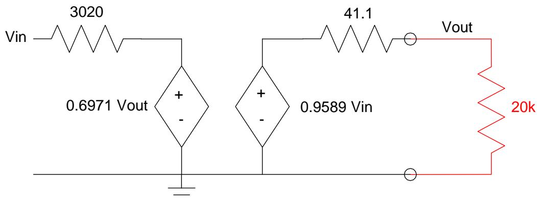
4) Determine the 2-port model for a 4-stage amplifier:
