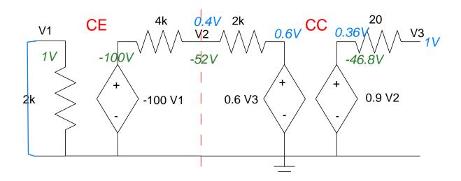
Rout: Short Vin. Apply 1V to Vout. Measure the current (shown in blue)
