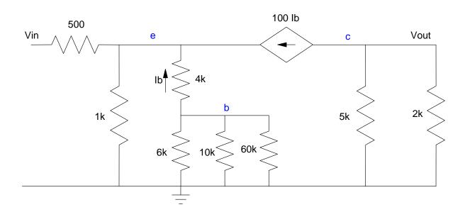
3) Find the 2-port parameters for the following circuit:
