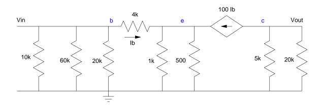
2) Assume the DC operating point is  $I_b=13\mu A$  (meaning  $r_f=4000\Omega$ ). Draw the small signal model for the following common emitter amplifier:
