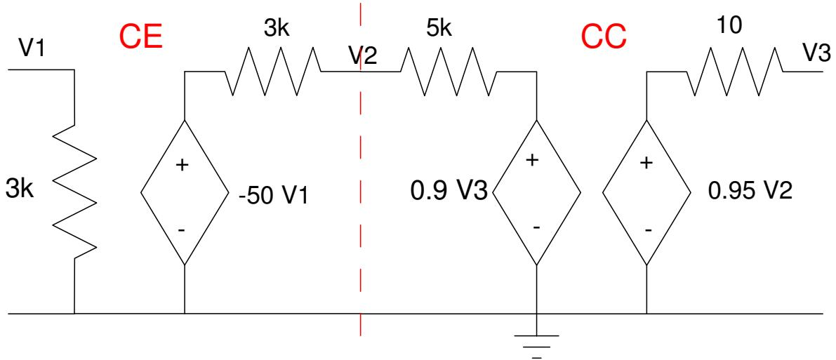
Rout: Short  $V_1$ . Apply 1V to  $V_3$ . Compute the current
