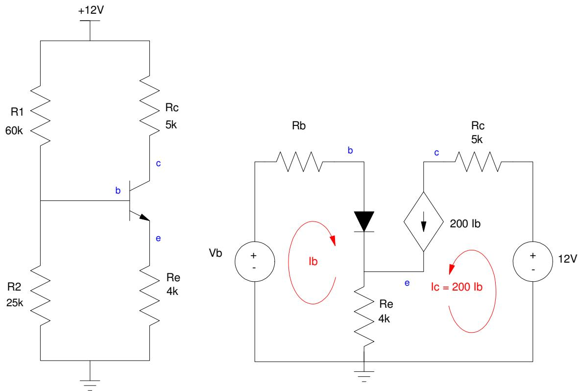
$$R_b = R_1 \parallel R_2 = 17,647\Omega$$
