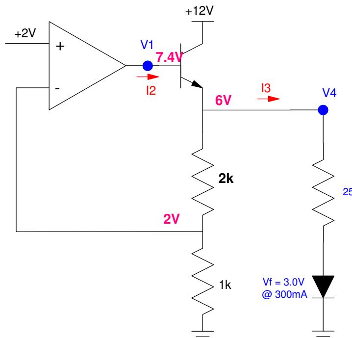
$V_+$  equals  $V_-$ . This means  $V_4$  must be 6V for  $V_-$  to be +2V
