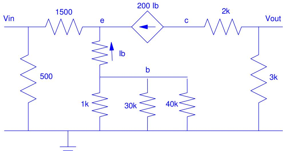
2) Determine the 2-port model for the following circuit.
