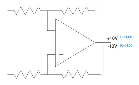
4) The following circuit uses a linearizing circuit with an instrumentation amplifier. Determine the voltages at V1..V4
