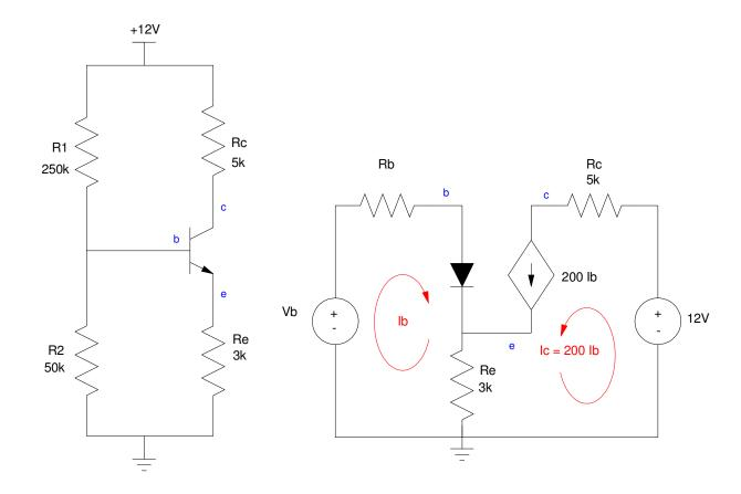
8) Draw the small signal model for the following common emitter amplifier (with Ce removed) and determine the corresponding 2-port model
