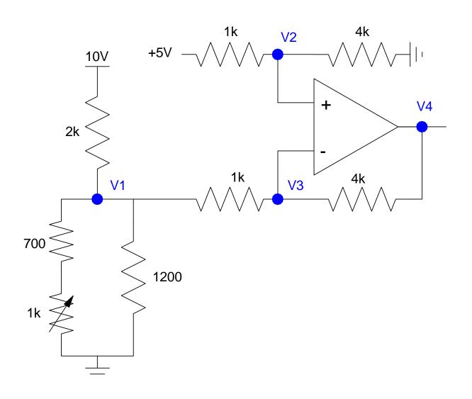
$$V_{2} = \left(\frac{4k}{4k+1k}\right) 5V = 4V$$
