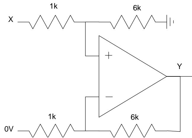
3b) Design an op-amp circuit with a gain of -6
