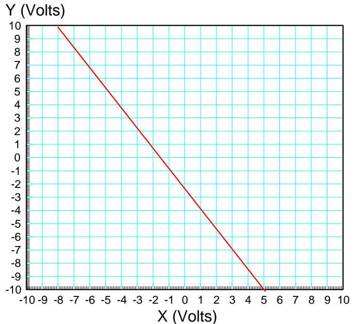
4b) Design an op-amp circuit to match the following relationship between X and Y:
