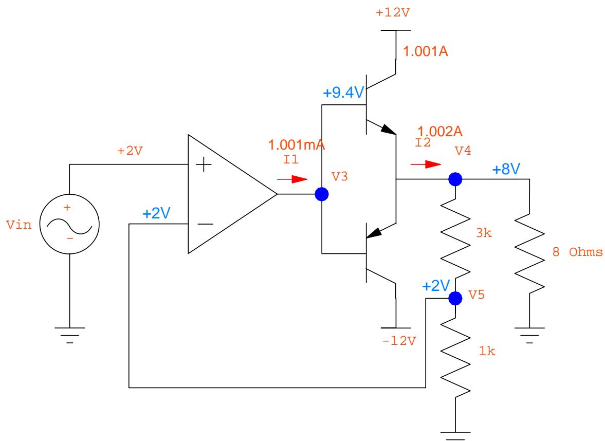
$$I_2 = \left( \frac{8V}{8\Omega} \right) + \left( \frac{8V}{4k\Omega} \right) = 1.002A$$
