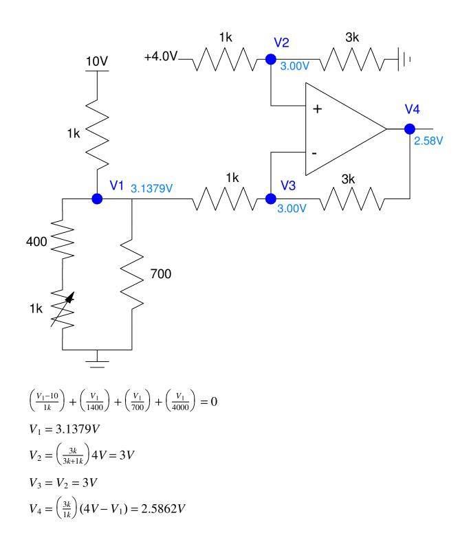
5) Let {A, B, C} be -10V to +10V analog voltages capable of driving 20mA (or less). Design a circuit to implement
