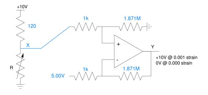
4) The following circuit uses a linearizing circuit with an instrumentation amplifier. Determine the voltages at V1..V4
