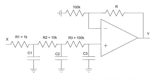
$$Y \approx \left(\frac{1 + \frac{R}{100k}}{(R_1 C_1 s + 1)(R_2 C_2 s + 1)(R_3 C_3 s + 1)}\right) X$$
