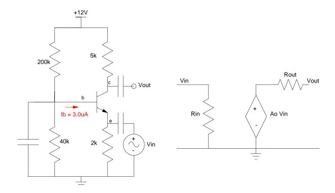
5) Multi-Stage Amplifier: Determine the 2-port model for the following 3-stage amplifier:
