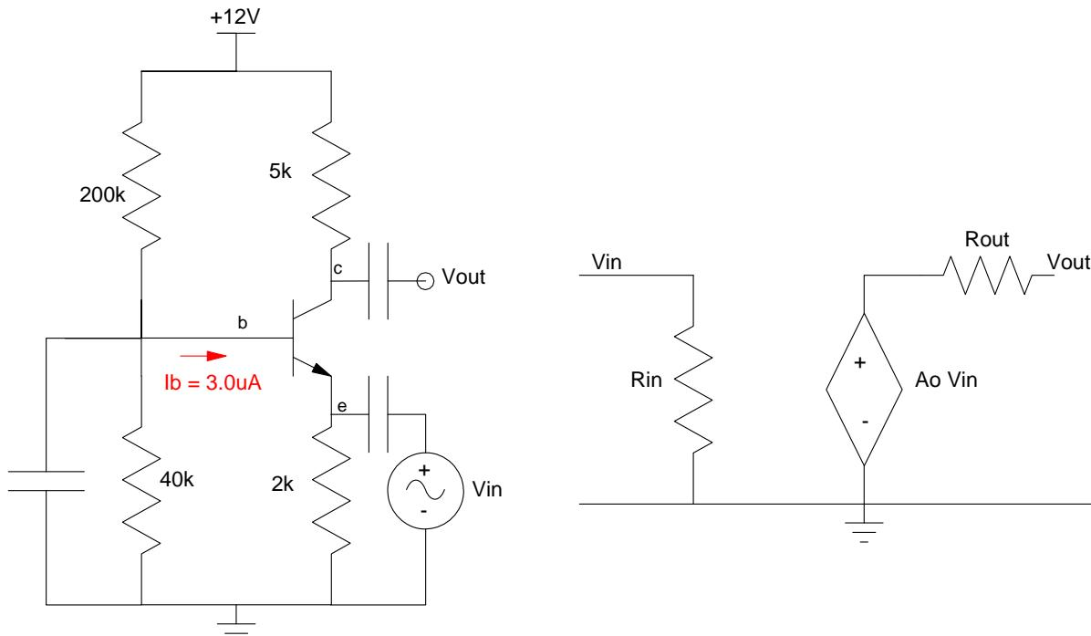
Rin: Apply 1V at the input, short the output, and compute the resulting current
