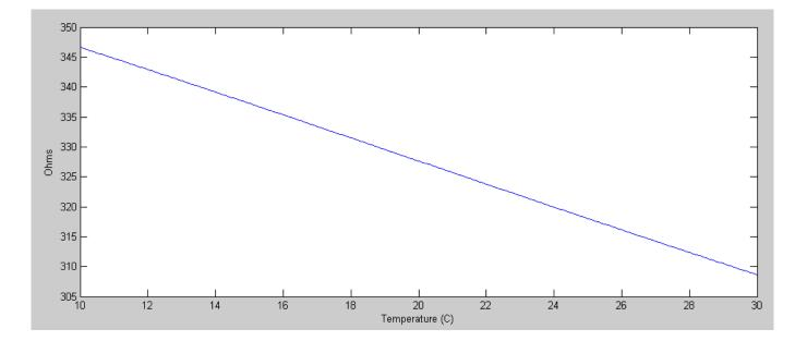
**Problem 2**) Using this linearizing circuit, design a circuit which ouputs -10V to +10V as temperature goes from 10C to +30C.
