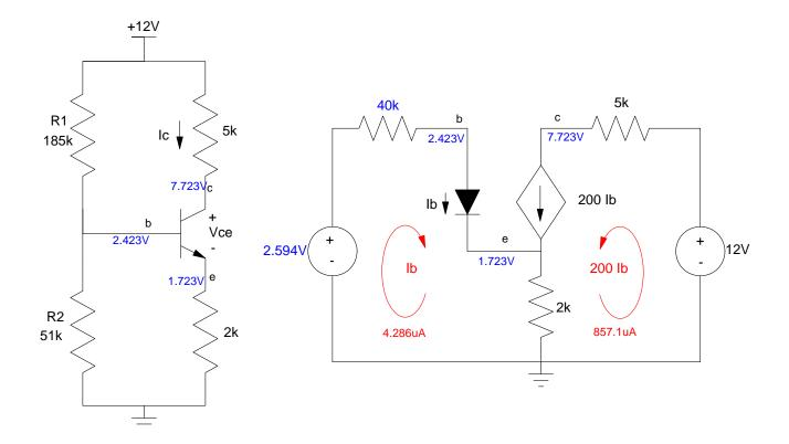
7) For your circuit of problem #6, determine the 2-port model for this transistor amplifier if set up as a Common Emitter amlifier
