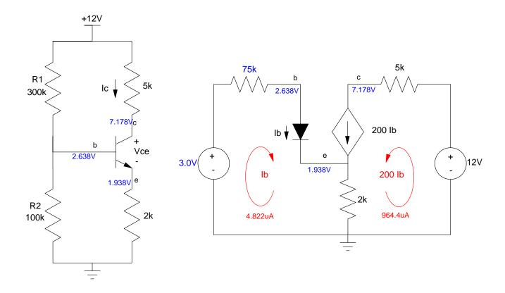
$$R_{b} = R_{th} = R_{1} ||R_{2} = 75k$$
