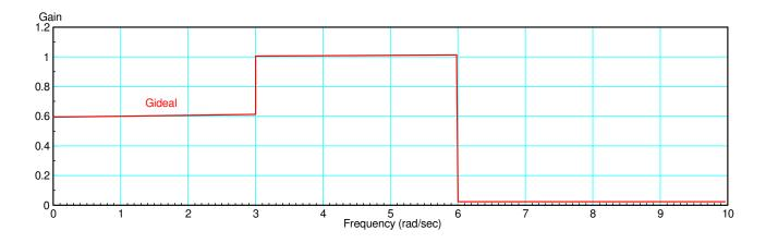
6) Filter Implementation: Design an op-amp circuit to implement the following filter:
