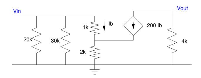
Rin: Apply 1V to the input. Compute the current
