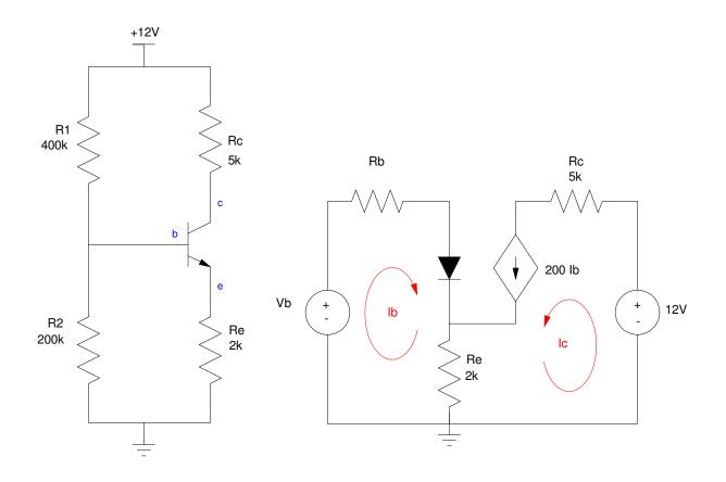
$$V_{b} = \left(\frac{200k}{200k+400k}\right) 12V = 4.00V$$
