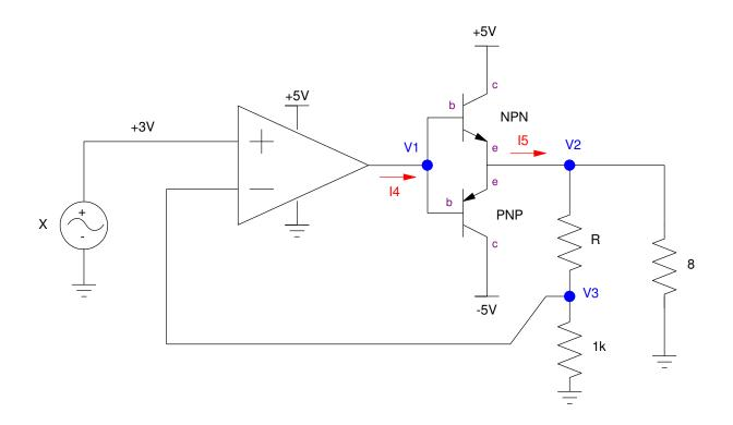
3) Push-Pull Amplifier: Current Output. Assume ideal silicon diodes and ideal silicon transistors with
