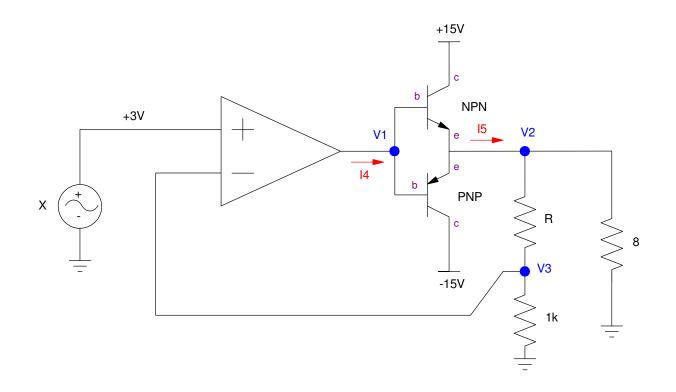
2) Push-Pull Amplifier: Voltage Output. Assume ideal silicon diodes and ideal silicon transistors with
