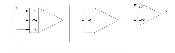
Adjusting the gains so they are all negative. Add an inverter when needed
