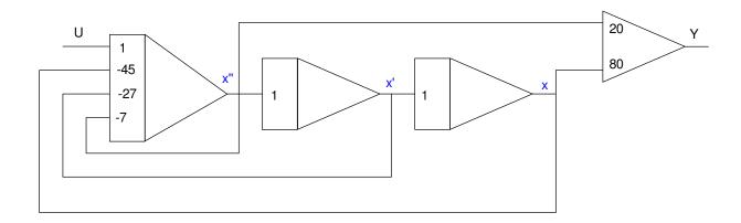
Adjust the gains so that they are all negative. Add an inverter (gain = -1) if needed
