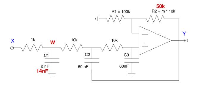
Note that this is an RC filter cascaded with an active low-pass filter
