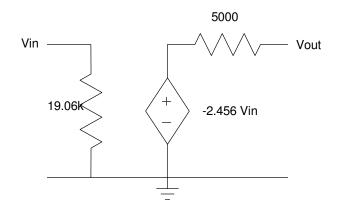
6) Simulate this circuit in CircuitLab. Verify each of the 2-port parameters at 1kHz Same simulation as before but with Ce = 1pF (essentially not there)
