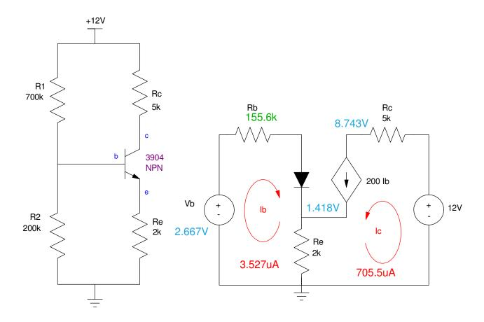
$$V_b = \left(\frac{R_2}{R_1 + R_2}\right) 12V = 2.667V$$
