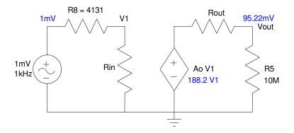
5) Remove Ce. Now draw the small-signal model for the circuit of problem #2. From this, determine the 2-port model for the Common Emitter amplifier
