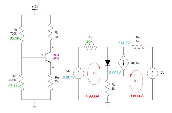
3) Draw the small-signal model for the circuit of problem #2 connected as a common emitter amplifier (below). From this, determine the 2-port model
