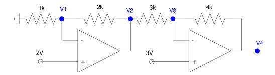
There are four unknown voltages, so we need to write 4 equations to solve for 4 unknowns. Start with the easy ones: at the output of each op-amp, V + = V-
