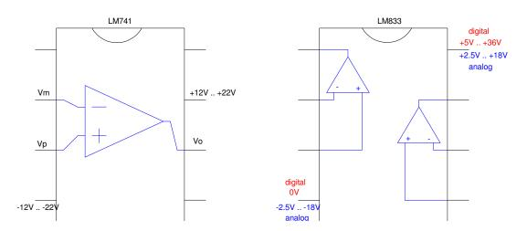
Pin Layout for two common op-amps: LM741 and LM833 The LM833 works for both digital electronics and analog electronics.
