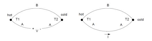
The Seebeck coefficient is a measure of the sensitivity of the thermocouple:
