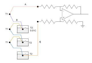
Several hundred such connections are often used in a single package. The exact number is often times not listed on the package, but can be derived based upon the sensitivity of the thermopile and sensitivity for a single connection given in the previous table.
