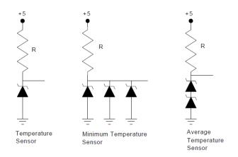
The resistor limits the current flow to the Zener diode. The voltage across the diode is then proportional to temperature.
