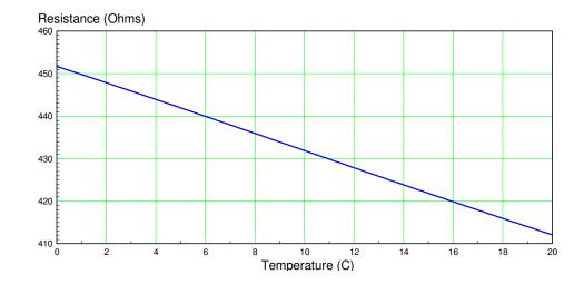
The advantage of using this linearizing circuit is that the resistance is much more linear than before. This makes calibration a simpler process (inverse log square functions don't need to be computed anymore). The disadvantage is that the sensitivity has been reduced. At 0C, the sensitivity is now -0.4%/C instead of -5%/C.
