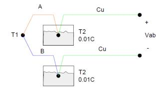
This law allows you to use a third metal in the thermocouple without altering the voltage or current, providing that both junctions are at the same temperature.
