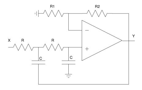
$$Y = \left(\frac{k \cdot \left(\frac{1}{RC}\right)^2}{s^2 + \left(\frac{3-k}{RC}\right)s + \left(\frac{1}{RC}\right)^2}\right) X$$
