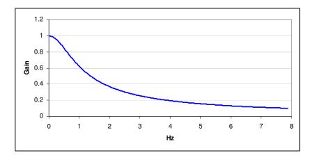
When the input is less than 0.5Hz, the gain is almost one: the output is almost as large as the input. When the input is past 2Hz (or so), the gain drops. In short, this filter passes low frequencies (near zero) and rejects high frequencies. Hence, it is called a low-pass filter.
