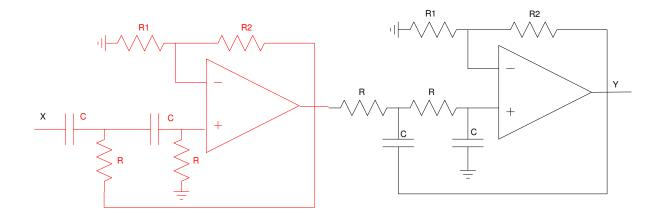
$\left(\frac{k \cdot \left(\frac{1}{RC}\right)^2}{s^2 + \left(\frac{3-k}{RC}\right)s + \left(\frac{1}{RC}\right)^2}\right)$
