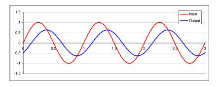
A simple way to relate the two signals is the change in amplitude and the phase shift.
