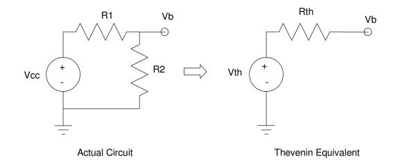
The idea behind Thevenin equivalents is this is a linear circuit: meaning the VI characteristics are a straignt line. Any circuit which has the same VI characteristic behaves the same as far as the output is concerned.
