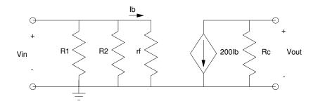
To simplify this, use a generic Thevenin equialent for a circuit with an input and output, termed a 2-port model:
