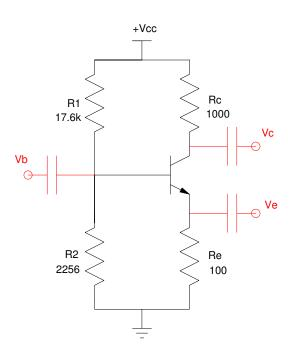
To prevent the outside world from messing up the Q-point, add capacitors to the base, emitter, and collector.
