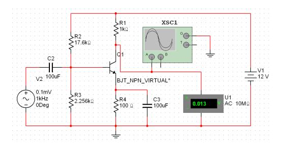
If you use DC coupling on the oscilloscope (left), you see the small AC signal at Vc riding on top of a 6V DC offset. If you switch to AC coupling to remove the DC offset, you can see the AC signal is 13mV rms, resulting in an AC gain of 130. The gain is supposed to be 115, so this is pretty close to our analysis.
