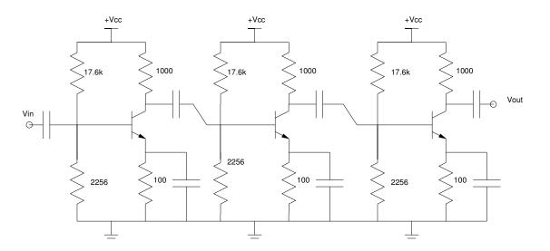
Solution: This is the same circuit we've been analyzing, copied three times. The 2-port model will be the same for all three sections since they're identical. Using the 2-port model then,
