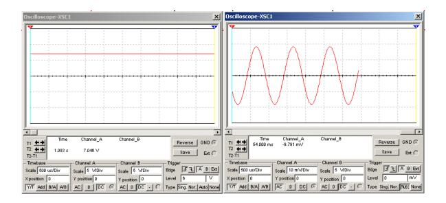
DC Coupling showing the DC offset of the Q-point (left) and AC coupling showing the gain (right)
