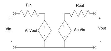
To find the two port parameters, come up with a test to find all four parameters for the 2-port model. Do the same test on the CE amplifier circuit.
