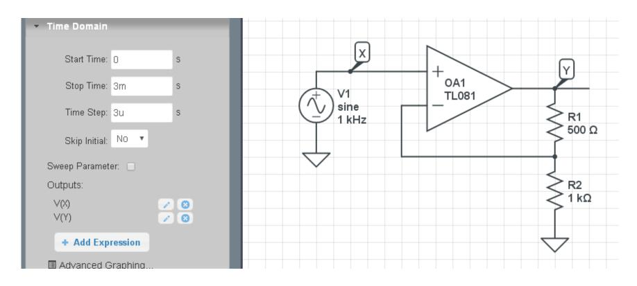
Running a simulation for 3ms (3 cycles) gives the following result.
