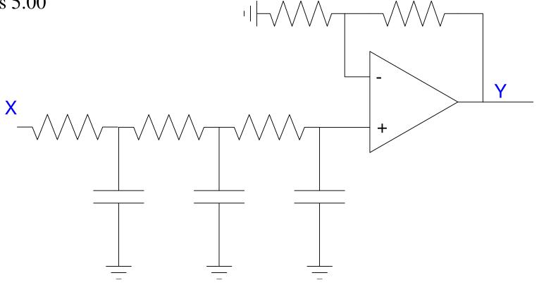
Option #2: Three 1st-order filters  $-Y = \left(\frac{-500}{(s+2)(s+5)(s+10)}\right) X = \left(\frac{-5}{s+2}\right) \left(\frac{-10}{s+5}\right) \left(\frac{-10}{s+10}\right) X$
