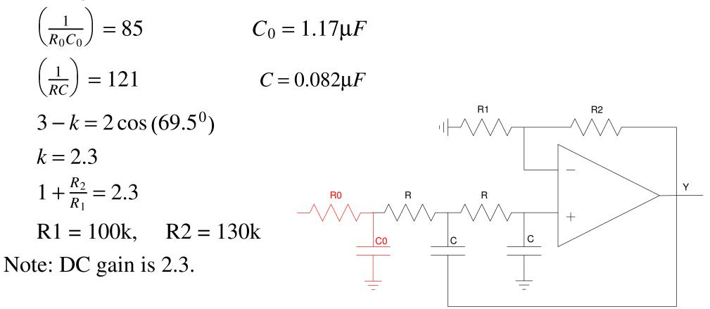
**Example:** Design a filter to implement  $Y = \left(\frac{100,000s^2}{(s^2 + 14s + 100)(s^2 + 100s + 10,000)}\right)X$
