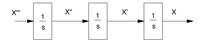
Step 4: Create X''' using the differential equation from step 2:  $s^{3}X = -(a_{2}s^{2} + a_{1}s + a_{0})X + U$
