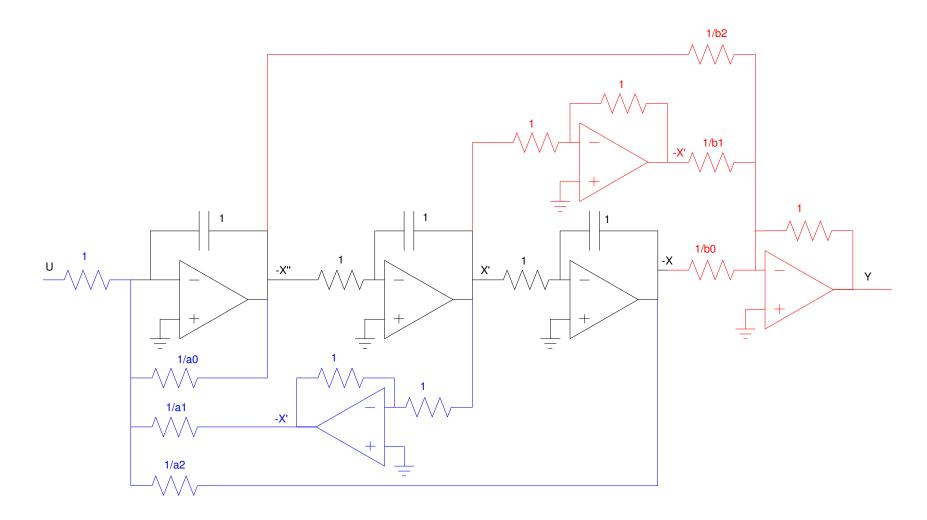
Final Op-Amp Circuit: All units M Ohms and uF.
