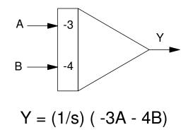
Applying this to the above block diagram:
