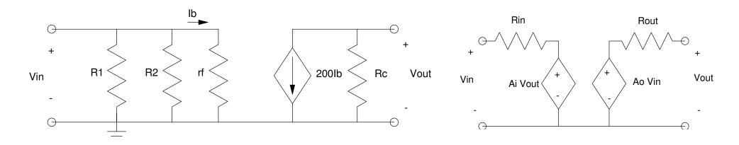
**Rout:** For the 2-port model, short Vi so that Vi=0 and  $A_oV_{in}=0$ . Measure the resistance at the output. Doing the same for the CE amplifier, this results in
