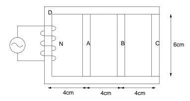
Determine the flux in each section of the core.
