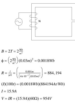
5) Assume the air gap is removed. The input is 240VDC, the resistance is 60 Ohms, and there are 100 turns. Determine a) the magnetic field intensity, b) the core flux density, c) the relative permeability of the core, and d) the reluctance of the magnetic circuit.
