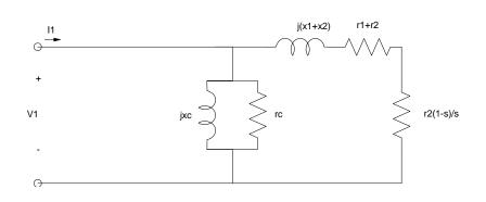
3) Assume a2-pole (ns = 377 rad/sec) single-phase AC induction motor operating at 120V rms. Assume the parameters are:
