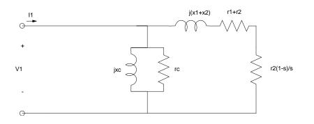
2) Assume you have a 2-pole (ns = 377 rad/sec) 3-phase AC induction motor with a line-to-neutral voltage of 120V rms and
