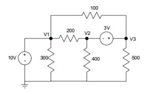
You need three equations for three unknown voltages. Start with the voltage sources:
